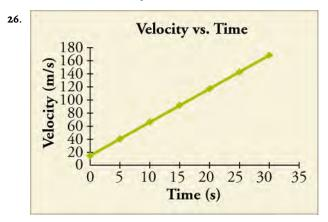
True or False: —The image shows a velocity vs. time graph for a jet car. If you take the slope at any point on the graph, the jet car's acceleration will be 5.0 m/s<sup>2</sup>.
